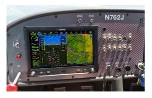
The Latest Technology- The J170-D is equipped with the most advanced avionics offered for light-sport aircraft. The standard-equipment Garmin G3X touch-screen flight display has intuitive controls and features synthetic vision 3D terrain, GPS moving map with the capability to display geo-referenced charts, AOPA airport directory, and a 2020-compliant ADS-B package with weather and traffic display. Full electronic engine monitoring, including 4-cylinder CHT, EGT, and fuel flow, is also standard.
