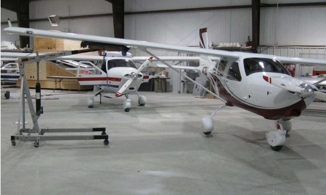
Figure 2-3: Jacking Aircraft with Engine Hoist
