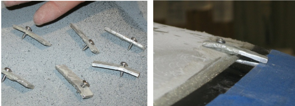
Figure 3-1: Window clamps made from 0.125" aluminum stock and sheet metal screws (left). Clamp in position holding upper portion of windshield to fuselage (right).
