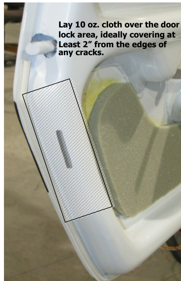
Figure 12-2: Door lock slot repair
