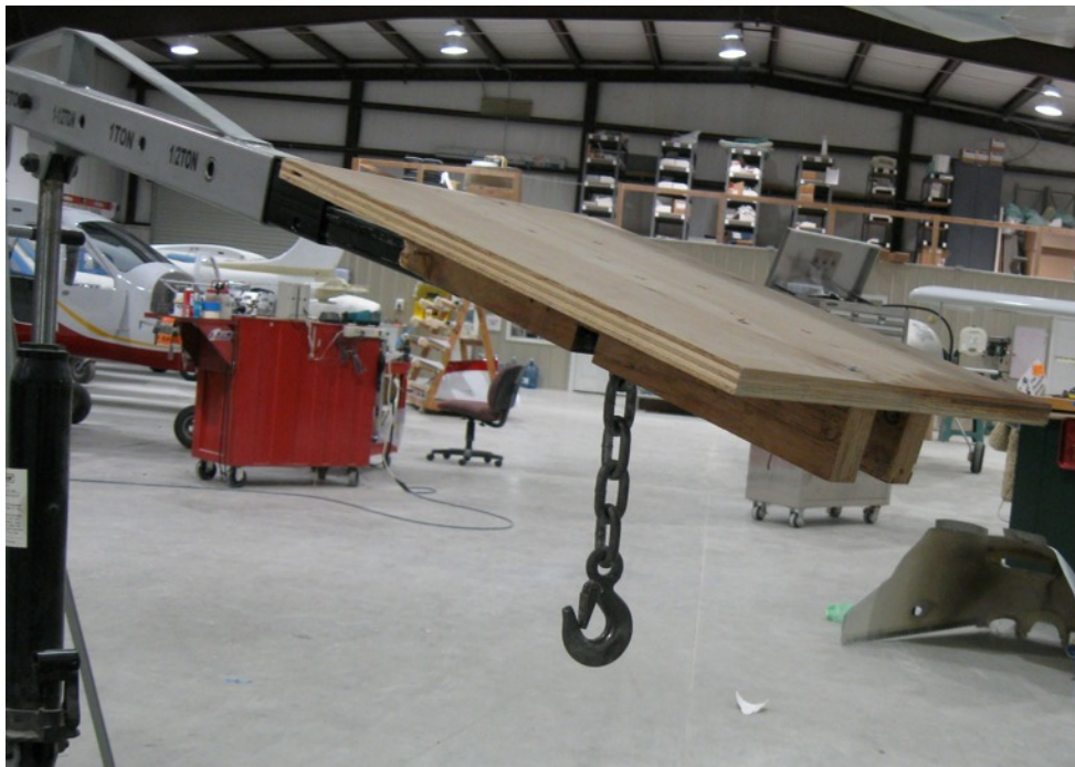
Figure 2-2: Plywood Jacking Platform on Engine Hoist
