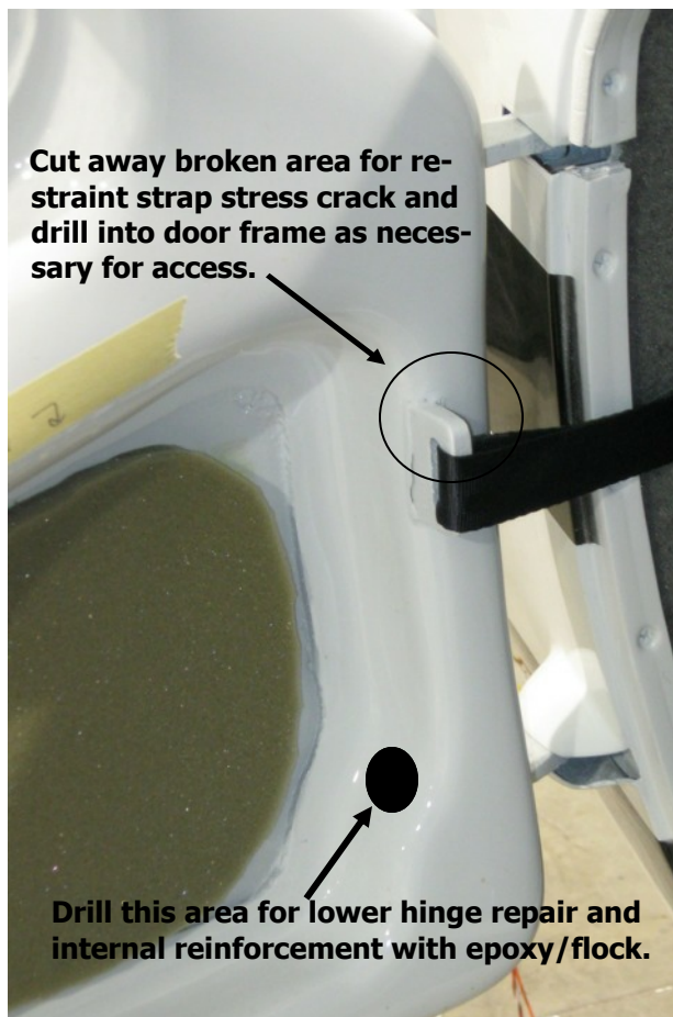
Figure 12-1: Hinge repair
