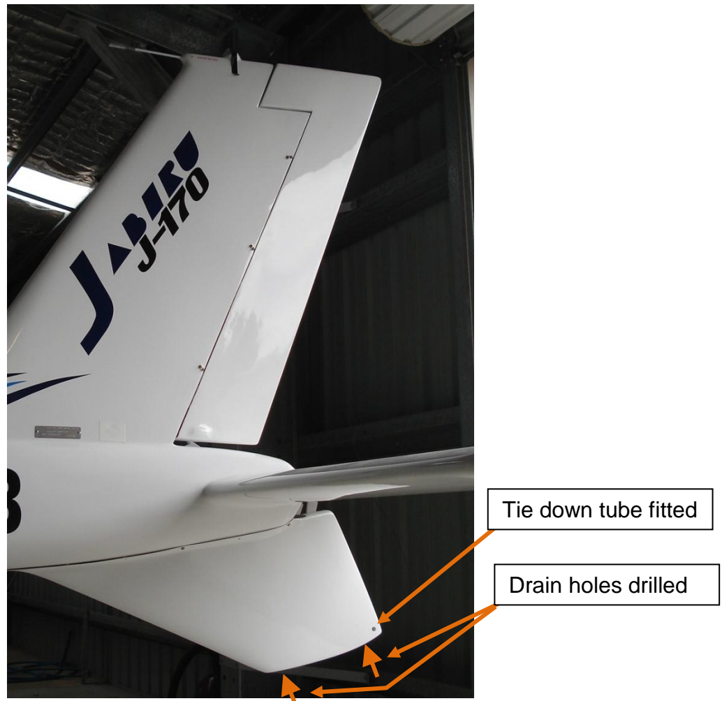
Figure 7 – New Ventral Fin Fitted
