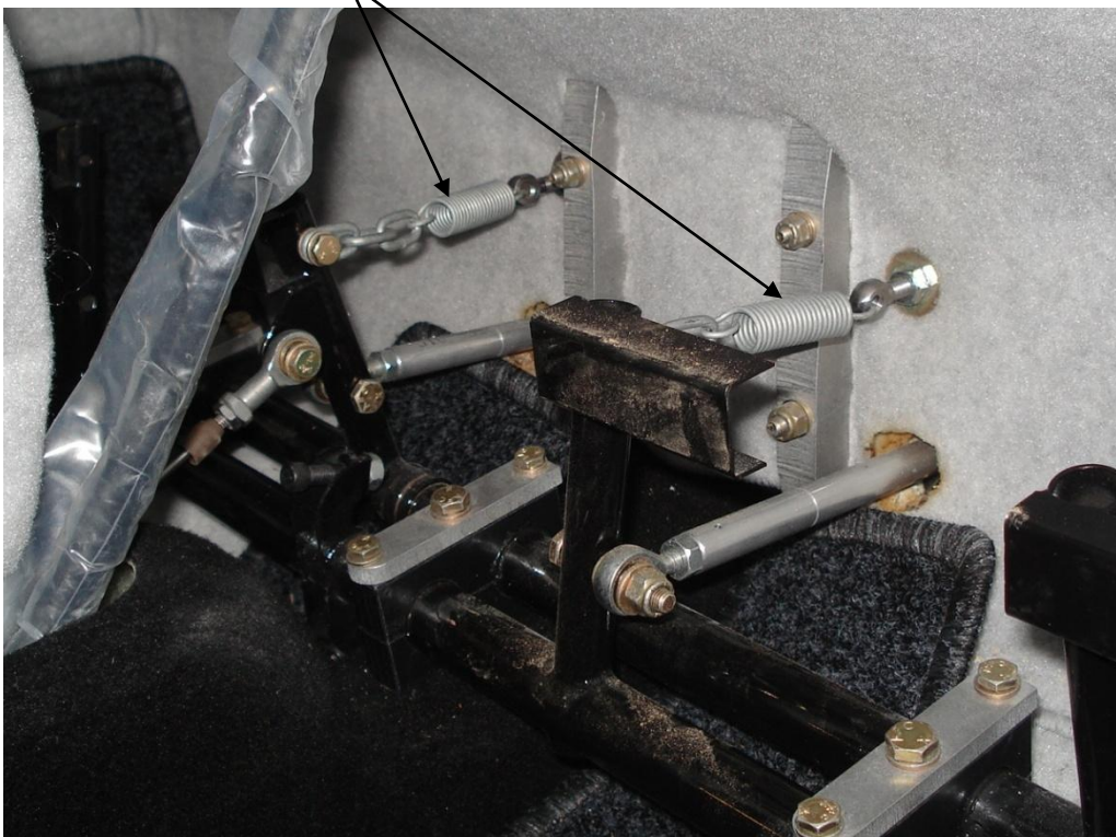
Figure 1 – Original Rudder Centring Springs
