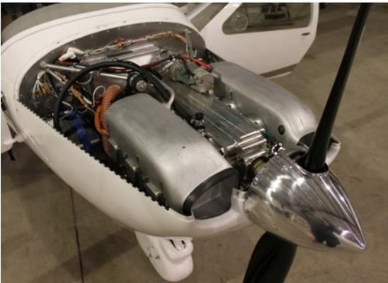
**Excellent Handling and Performance**—The generous control surface area combined with ergonomic controls make the Jabiru a delight to fly, even on windy, bumpy days that will keep the pilots of other LSAs at home. Inherent stall/spin resistance enhances safety. The 120-horsepower, direct-drive, 6-cylinder Jabiru 3300 offers more power and smoother operation than the competition and features the latest Jabiru safety enhancements.
